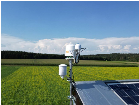
Figure 9: ASI 16/55 on the roof of a greenhouse in Illemad, the neighbouring village. In the foreground, a pyranometer for measuring global radiation is visible, as well as a ventilated radiation shield on the left, which protects a sensor for measuring air temperature and humidity from direct sunlight.
