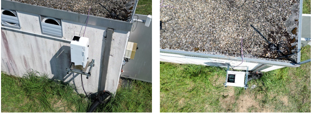
Figure 11: SkyVue8 lidar ceilometer installation at the Buttenwiesen I site. The device is mounted on the exterior wall of the measurement container to monitor cloud base height and vertical aerosol profiles. To mitigate potential damage from wildlife, the device was installed in an elevated position.
