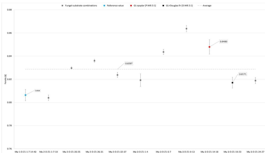
Figure 9. Porosity results of the examined fungal-substrate combinations.
