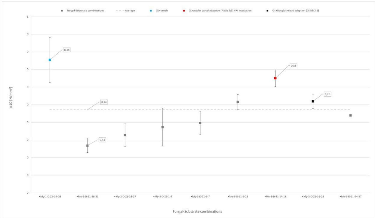
**Figure 7.** Compressive strength comparison among all fungi-substrate combinations.
