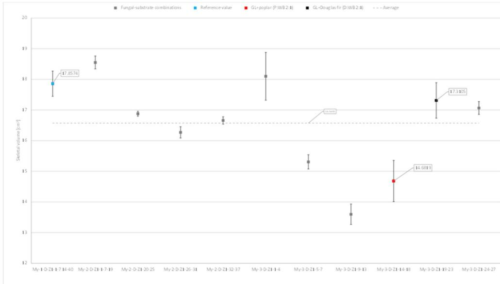
Figure 7. Skeletal volume results of the examined fungal-substrate combinations.
