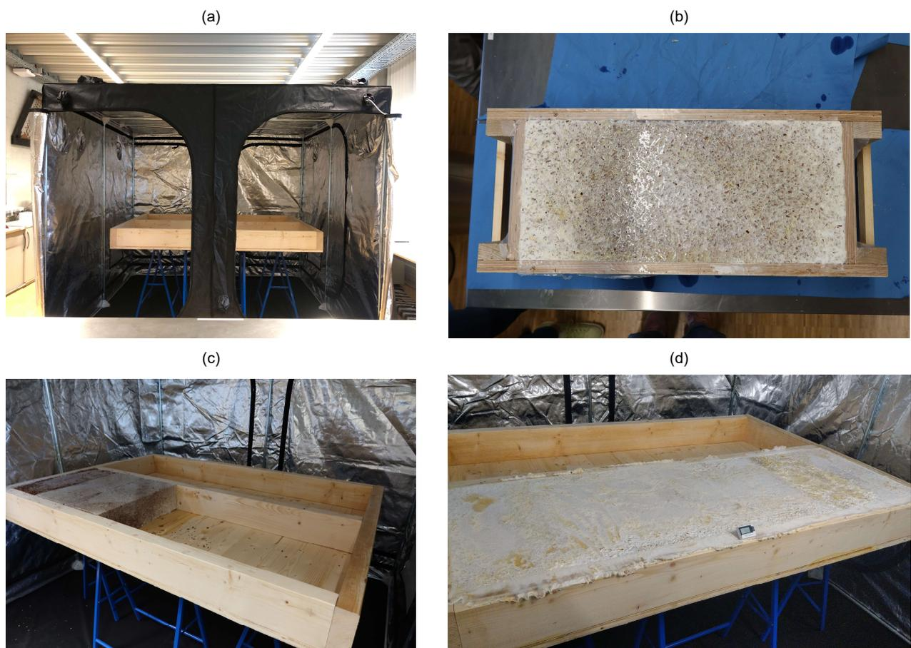
**Figure 11.** (a) wall prototype in scaled up incubator (indoor growing tent); (b) module A in formwork after two weeks of incubation; (c) installation of MBC into the frame; (d) cultivation monitoring after three weeks.
