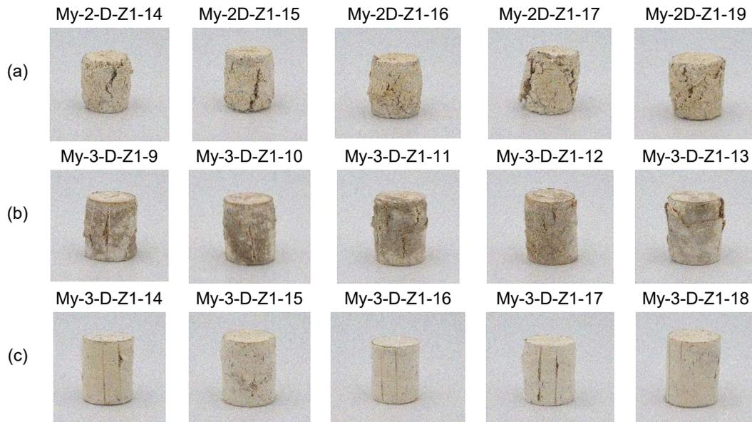
**Figure 9.** (a) Beech samples, (b) Poplar samples (with P:K 10:1), and (c) Poplar samples (with P:K 2:1). All pictures were taken after 20% strain.
