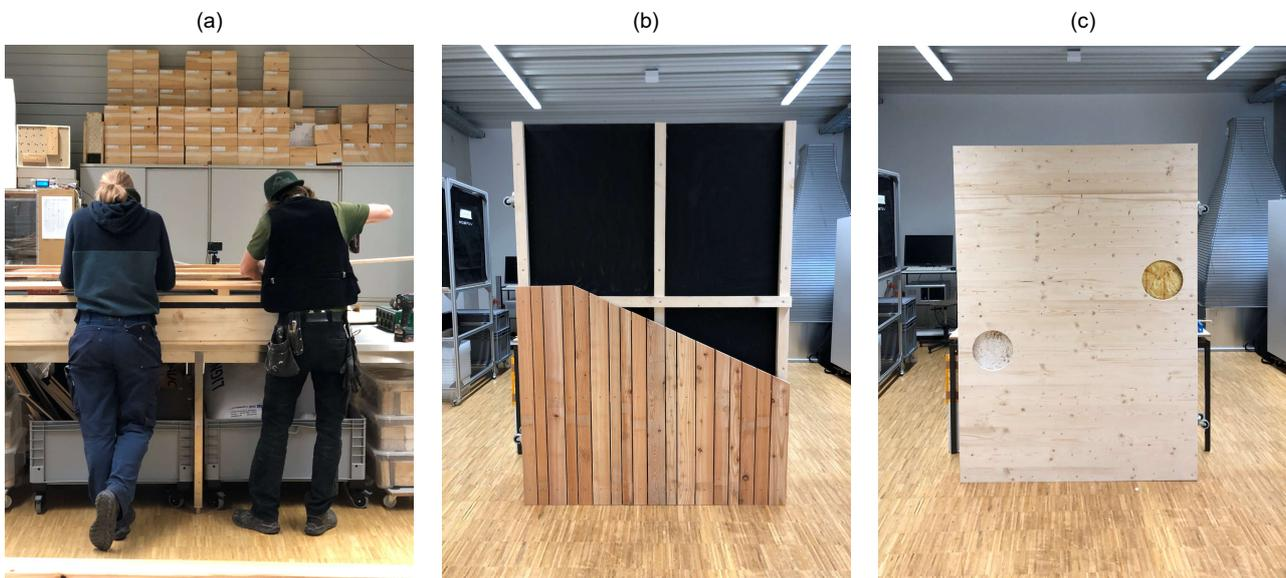
**Figure 12.** (a) project partner team finishing up the wall, (b) façade with larch cladding; (c) interior side of the wall with two controlling openings.
