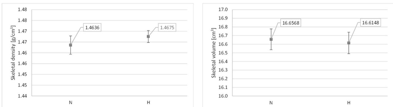
**Figure 6.** Comparison of skeletal density (left), and skeletal volume (right) measured with N, and H.
