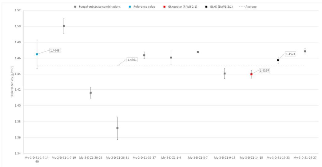
Figure 8. Skeletal density results of the examined fungal-substrate combinations.
