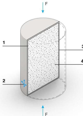
**Figure 8.** Illustration of the jacket effect of the quasi-pure mycelium surface on the poplar samples where  $[\rho_1 > \rho_2]$ . (1) Binding are between myco-jacket and MBC; (2) activation of the axial stresses alongside the myco-jacket surface (3);  $\Phi_1, \rho_1$ ; (4)  $\Phi_2, \rho_2$
