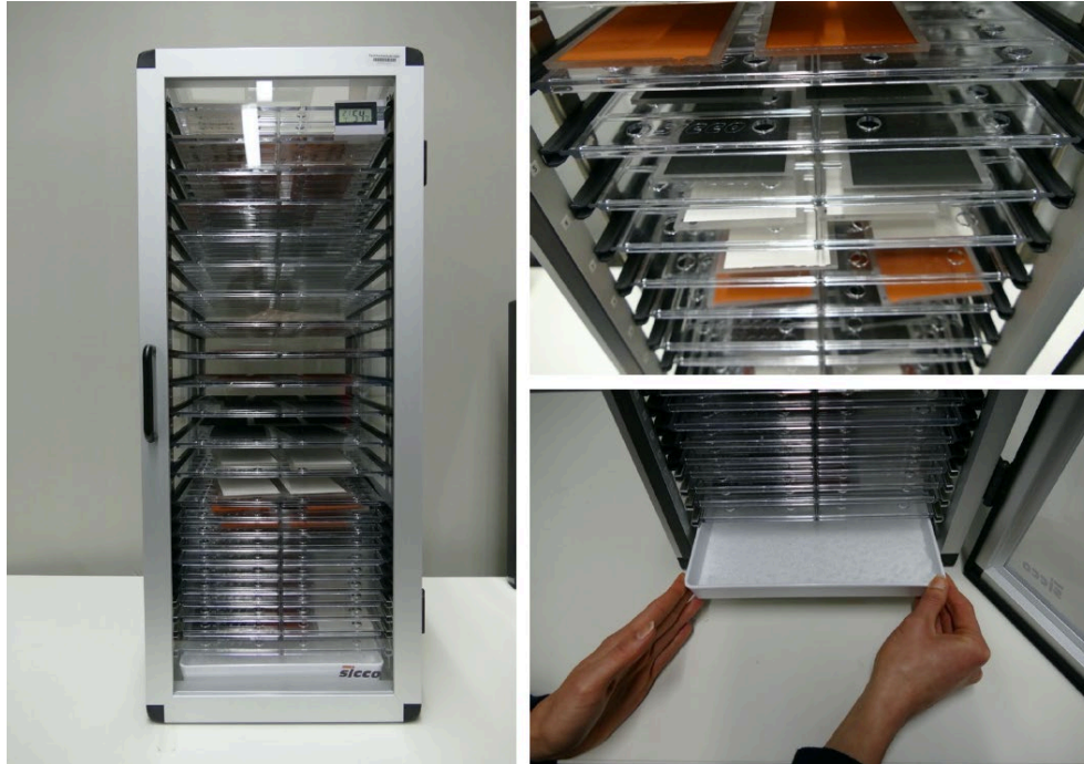
Fig. 7: Mock-up storage system Sicco tower. A tray with magnesium nitrate saturated solution guaranteed a stable environment (54% RH) in a climatized room (Temperature 22 °C)
