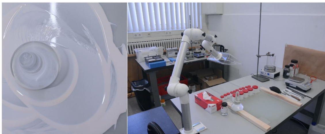
Fig. 3: Setup for mock-up paint preparation.
