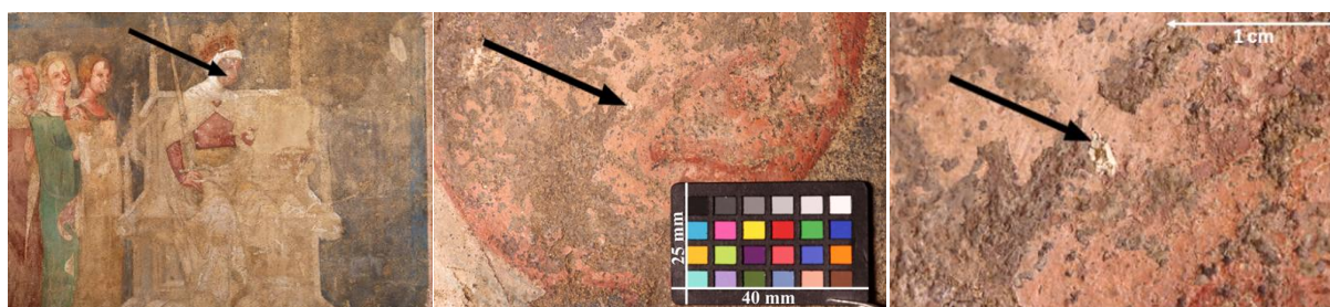
Figure 63: Photographic documentation and localisation of sampling: Judith's face, scene Judith with the Head of Holofernes, Bay 5(5), from the left: location of sampling pointed in a photogrammetric image (©Jiří Vidman); detail with a reference colour chart which also serves as a scale (©Vojtěchovský, Jakubů, Lesniaková); macrophotography with a scale (©Jan Vojtěchovský, Daniela Jakubů, Petra Lesniaková).
