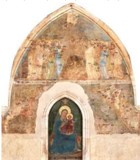
Figure 31: Example of the strategy of pXRF measurements on bay 25 (32). Photogrammetric image © Jiří Vidman, Pavel Hlavenka.
