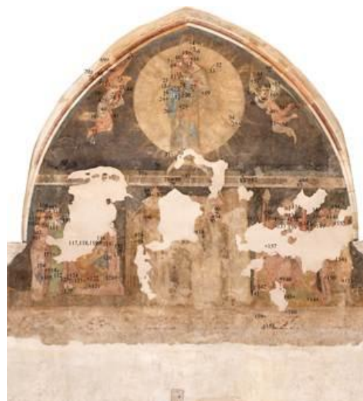
Figure 32: Example of the strategy of pXRF measurements on bay 6(6). Photogrammetric image © Jiří Vidman, Pavel Hlavenka.
