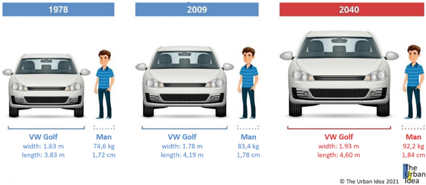
Fig. 1. The size growth of passenger cars using the example of the VW Golf [4].
