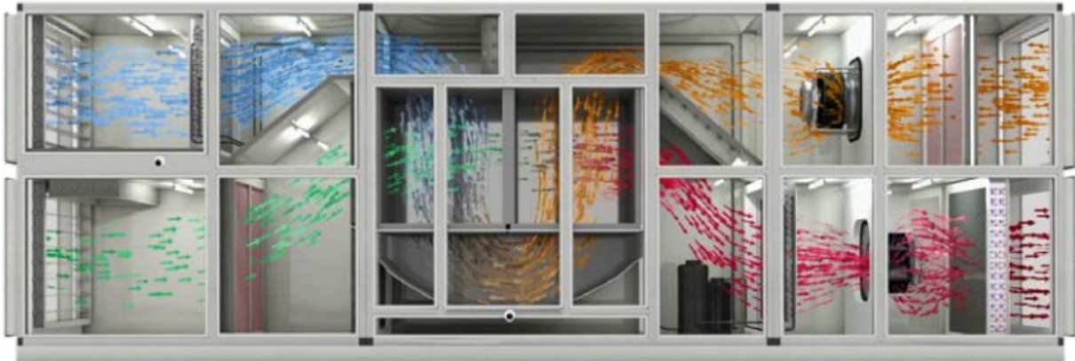
Figure 31 Partial Recirculation in winter mode
