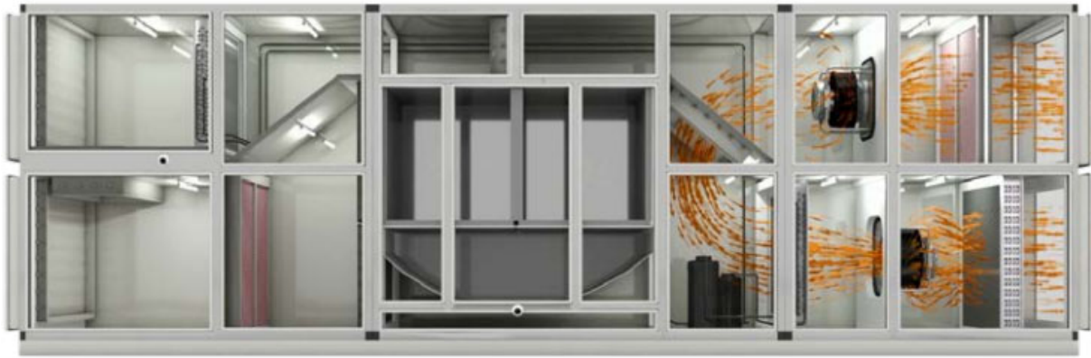
Figure 3 Recirculation without dehumidification
