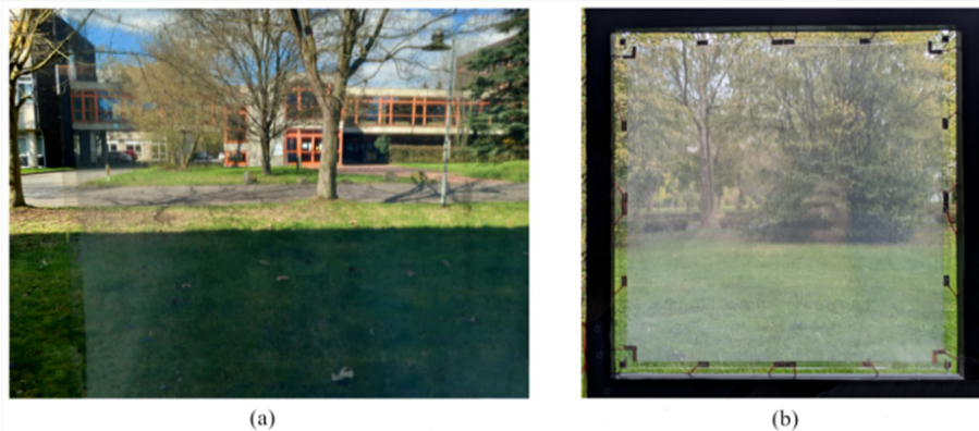
Figure 6. Images of a (30×30) cm 2 sample: (a) View through a MEMS micromirror array after fabrication. (b) Window module (double insulation glazing, argon, spacers, butyl sealing) with integrated MEMS micromirror array. The mirror status is partially closed. Contacts for subfield addressing are visible (2×2 subfields).
