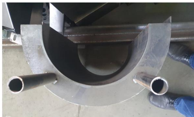
Figure 4.13 Steel mould for the fireclay mantel
