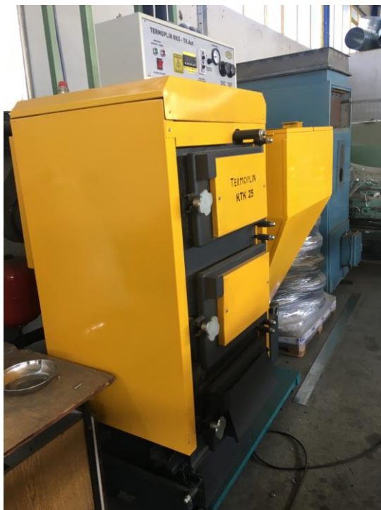
Figure 4.8 Combustion test stand in Termoplin
