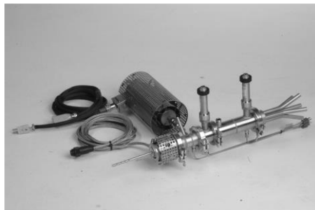
Figure 5.5 Sampling probe with heated primary dilution air (FPS manual full 5.8)
