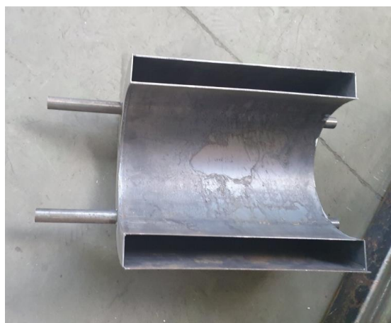
Figure 4.12 Steel mould – top view
