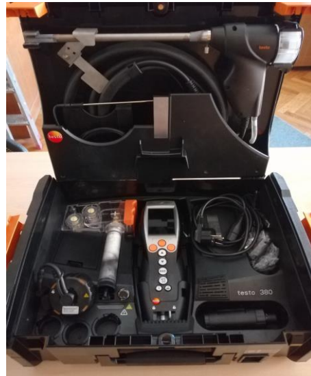
Figure 4.2 The newly purchased TESTO 380 for \text{CO} , \text{O}_2 and PM measurements
