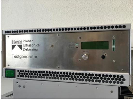
Generator: 1000 Watt / 18 kHz / 20 kHz
