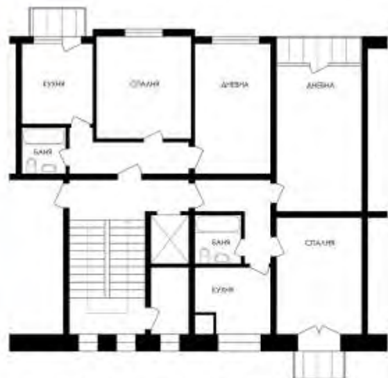
Sofia, 59 "Skobelev" Blvd. Plan of the corridor type apartments from a residential block. 1952-1954
