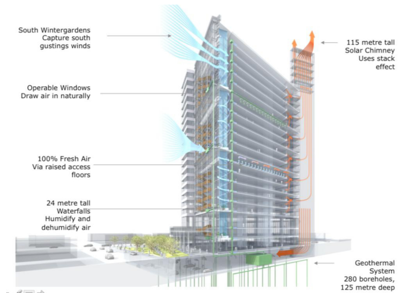
fig. 45: summer school 2014 Prof. Thomas Auer „Climate-Responsive Building Design“ Manitoba Hydro Place Energetic concept in Winnipeg
