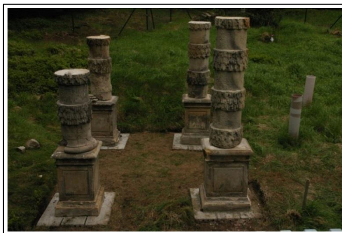
Fig. 14: Four test columns at the research station: anticlockwise starting right in front: Frühling (fabric), Sommer (light-weight), Herbst (wood) and Winter (without covering).
