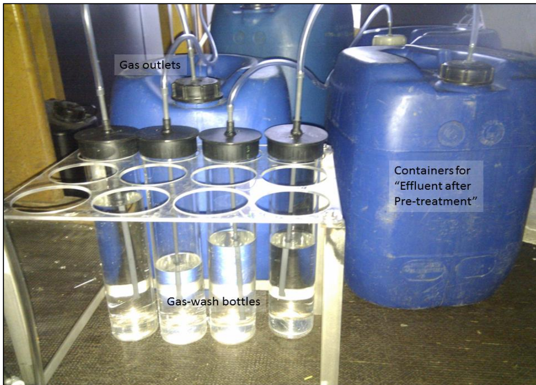
Figure 9: Setup for the acidification process carried out before the first prototype trial using "effluent after pre-treatment".
