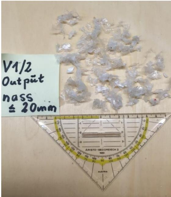
Abb. 18: Output nass Material <20 mm Flakes
