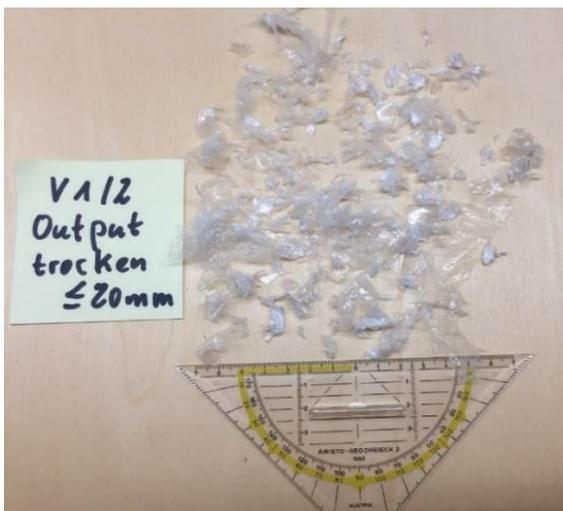
Abb. 20: Output trocken Material <20 mm Flakes
