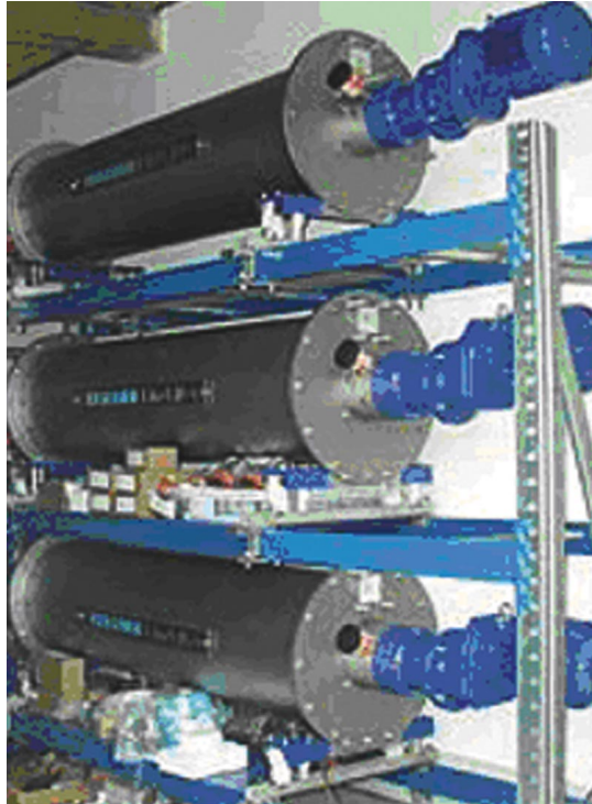
Figure 11. Rotating disc filter: Bellmer Fine Filter
