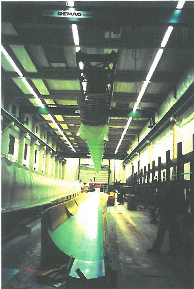
Rovingtransfer mittels langer Traverse
